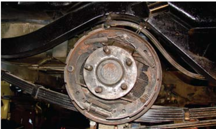
Corvette racing historians didn't know until they saw this six-leaf rear spring, complete with experimental part number, that the suspension system at Sebring was different from the RPO 684 package.
