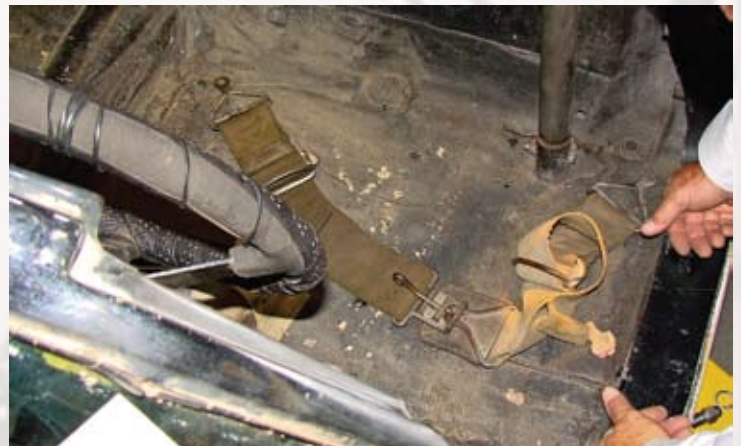
Date coded safety belt looks like military issue. Notice the roll bar mount. The bar is a modern design meeting SCCA slalom requirements in the '80s, but the mount is original.
